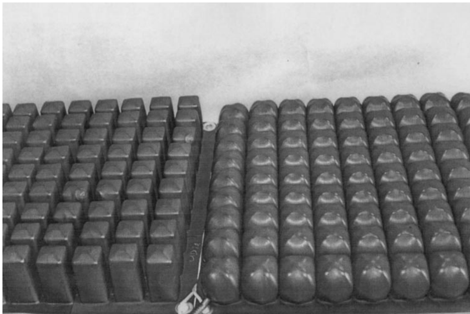
Figure 1. The two cushions shown are of the pyramidal air sac profile. The cushion shown on the left is the 75-mm high, square air sac model (cushion 4), and shown on the right is the 50-mm high, pyramidal air sac model (cushion 2).
